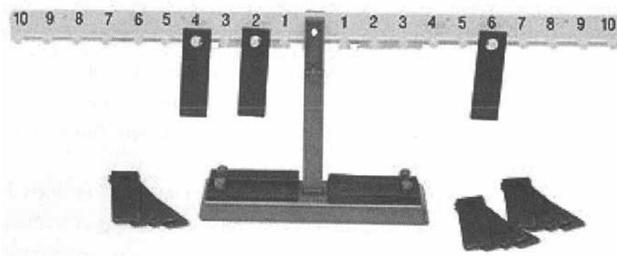
The mathematical scale is equal when the graduated beam is horizontal. Here, two plaques are respectively placed on the graduations 2 and 4 equalling having a plaque on the graduation 6 (Celda©).
