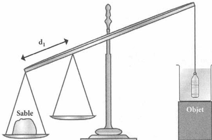
When the object is plunged into water, its weight diminishes, the balance is not equal.
