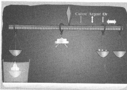
Extract from the animation: there is a relation between the distance between the two receptacles on the right and the material which makes the submerged object (on the left). This depends on the apparent weight of the immersed object, that is to say its volume mass.
