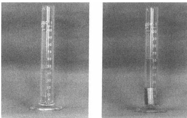
You can measure the volume of a solid in whatever shape or form by using a graded test tube: the volume of water in the test tube corresponds exactly to the volume of the object.
