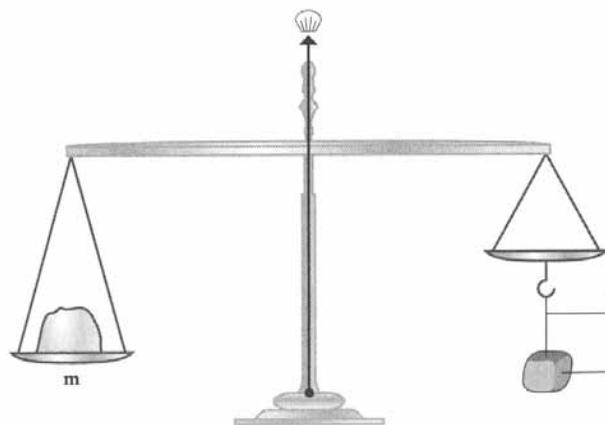
When the balance beam with receptacles is horizontal, the weight of the bowl is equal to a certain quantity of sand.
