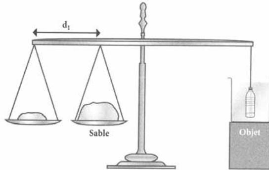
To re-level the balance, it is necessary to move a certain quantity of sand from the sachet furthest left to the right-hand sachet.
