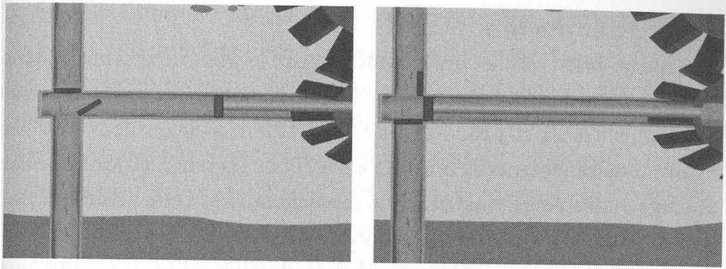
This animation extract shows the piston rotating by the slider crank mechanism. When the rod moves backward (left drawing), the first valve opens and lets the water from the river flow in by way of suction. The forward movement of the rod pushes back the piston, causing the valve to close (Right drawing). The water is then pushed backwards, leading the second valve to open, causing the water to flow upwards into the upper pipe, under the pressure of the piston.
