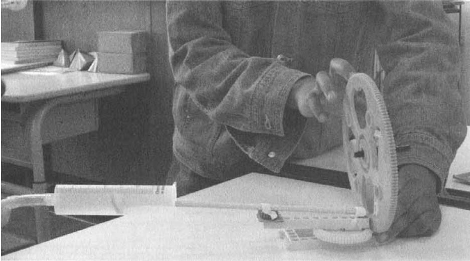
The rotation movement of the horizontal wheel ( crank wheel) is obtained thanks to that of the vertical wheel (driving wheel)
