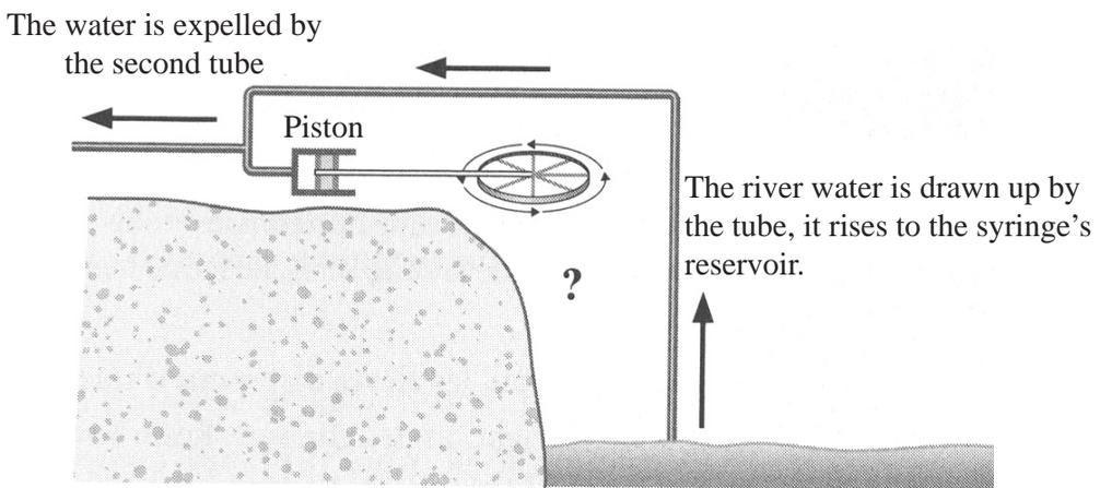
Here, the wheel is not vertical, (see the two preceding illustrations), but horizontal. In the same way as in the preceding example, the movement of the wheel's rotation makes the coming and going movement of the piston. It is now necessary to add a second wheel, this time vertical. This is what will drive the horizontal wheel due to the current of the river.
