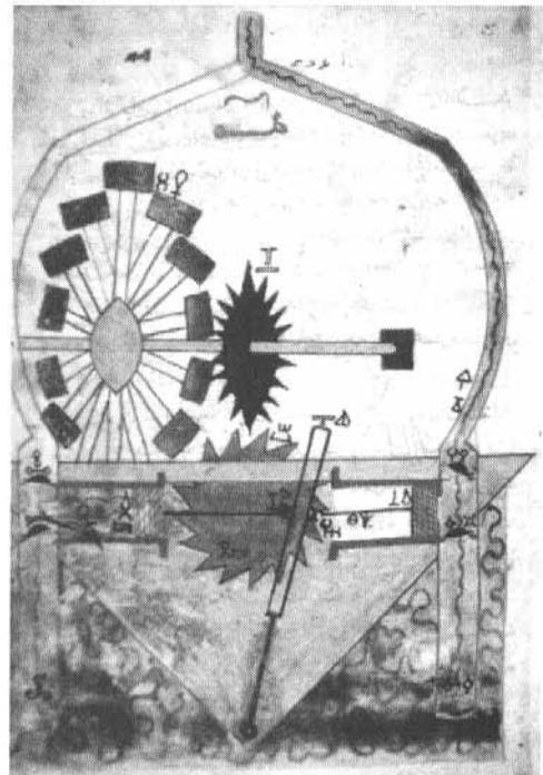
The working of this sucking and exhaling pump can be described as follows. The fixed blade wheel at the end of a horizontal beam is powered by running water. In turning, it powers the toothed wheel placed at the other end of the beam. The teeth of which enmesh with the teeth of a crank-pin disc placed at the end of a beam parallel with the first. The fixed crank-pin on the toothed disc
