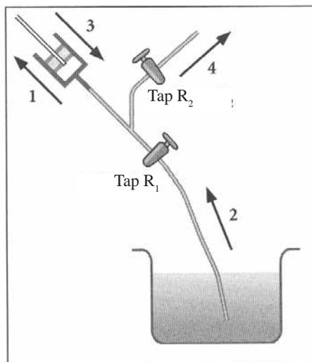
At the end of this activity, the pupils understand that the drawn water depends on the coming and going movement made by the piston of the syringe. We still have to find the means to do this without human intervention.
